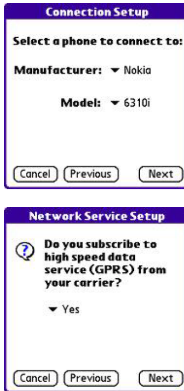
Figure 3 Steps to Pair a Palm Tungsten T with a Nokia 6310i
