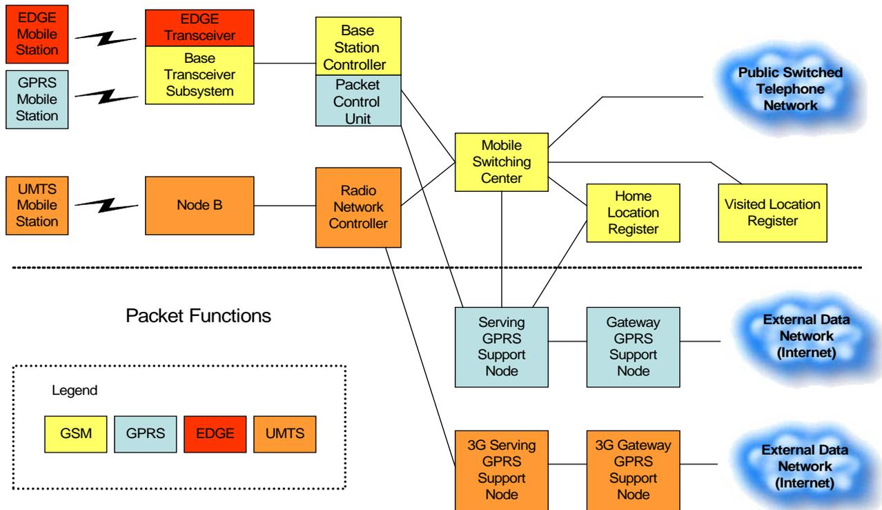
The biggest difference between GSM/GPRS/EDGE networks and UMTS networks is in the radio access network. UMTS uses a wideband CDMA radio interface that is described in the next section. However, the structure
